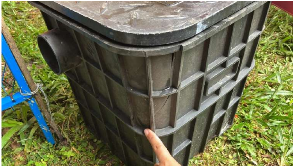
Photo 25: An approximately 15cm crack (half of the height) causing the item to be defective and unable to use.
